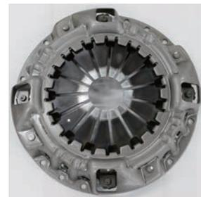
In most cases, the clutch cover is integrated with the pressure plate. Since the pressure plate is a degradable item, it must be replaced periodically. During a clutch disc replacement, make sure to inspect the clutch cover and recommend to your customer that this be replaced as well.
