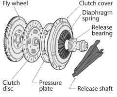
Fig. 2 Clutch construction
